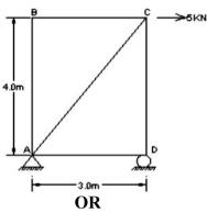
b) For the truss shown in Fig, find the member forces using method of 13, K2,CO6 joints.
