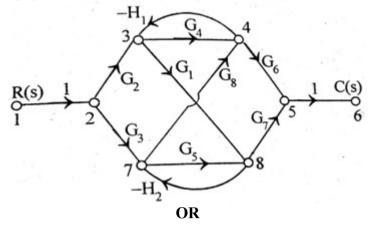
b) Evaluate the transfer function of the system by reducing the given <sup>15</sup> K<sup>3</sup> CO2 block diagram.
