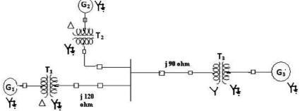
Construct the impedance diagram and mark all values in p.u choosing a base of 30MVA, 6.6kV in the generator 1 circuit.
