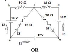
b) Infer the mesh currents in the circuit shown below.
