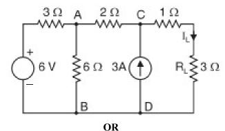
b) Solve the current in various resistors in the circuit shown in fig. by converting 10 K3 COI voltage sources into current sources.
