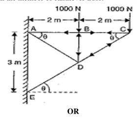
b) Analyze and predict the forces in all members of the truss shown in figure by using 11 K3 CO6 any one analytical method.
