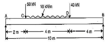
b) Draw Shear Force Diagram and Bending Moment Diagram for the overhanging 11 K3 CO3 beam shown below. Also locate the point of contra flexure.
