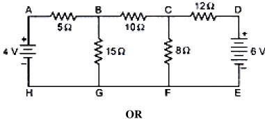
b) Determine the current flowing through branch I<sub>L</sub> of the given network Fig. using 11 K3 CO2 Norton's theorem.
