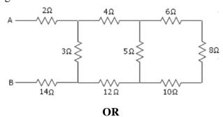
b) For the electrical network shown in Fig. determine the loop currents and all branch 11 K3 CO1 currents.
