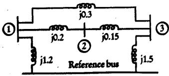
26. a) Figure below shows a simple power system network. Construct the positive, 11 K3 CO4 negative and zero sequence networks. The numerical data of various components in the power system is given as under: (all values are in p. u.)
