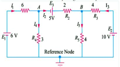
K3 CO2 24. Make use of Norton's equivalent circuit and solve for load voltage and load current.
