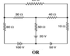
K2 CO1 b) Show the branch currents of the network by using mesh analysis or Nodal analysis.
