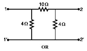
b) Determine the Z-parameters of the T-network shown in Fig. Also express the parameters of T-network in terms of Z-parameters.
